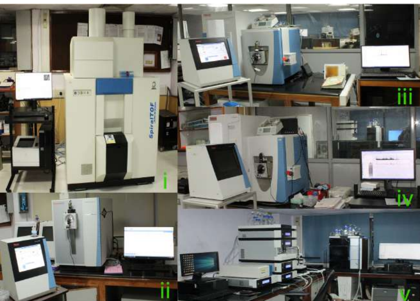
Left image: i - JEOL Spiral TOF JMS-S300, ii - Thermo Scientific Orbitrap Exploris 240, iii - Thermo Scientific Q Exactive HF, iv - Thermo Scientific Q Exactive, v - Thermo Scientific Dionex Ultimate 3000
